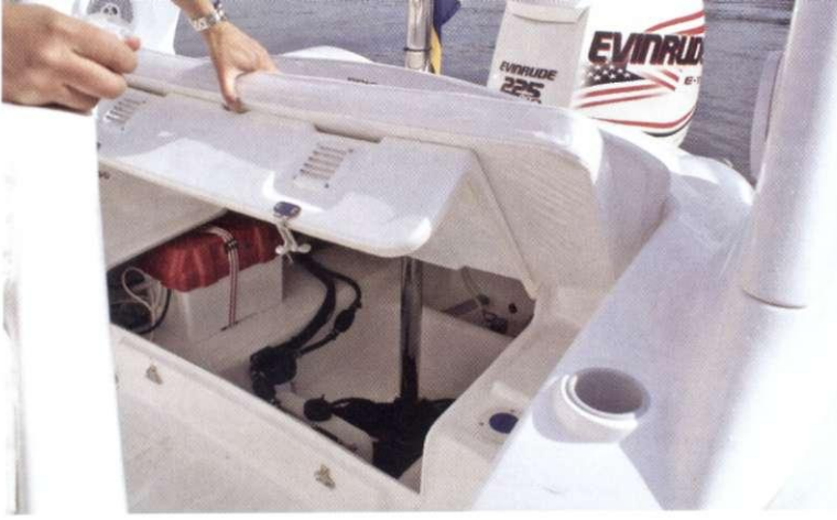
Above: The compact rear lounge flips up for bilge access. Note removable ski pole.
